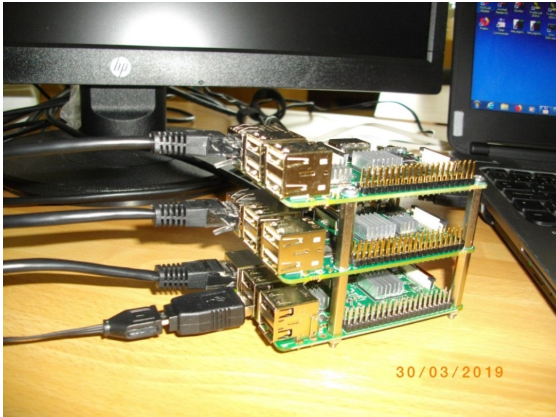
Figure 19: Two ZynqBerry boards and RPi3
