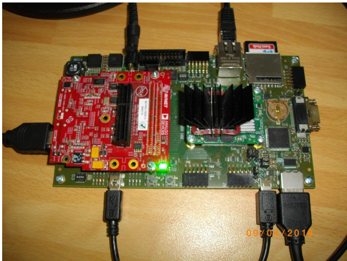
Figure 20: TE0820-03-4EV-1E on TE0701-06, Imageon HDMI I/O FMC card
