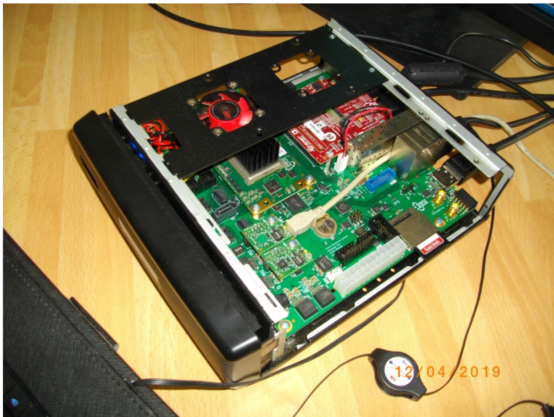
Figure 22: TE0808-03-15EG-1EE on TEBF0808-04 and Imageon HDMI I/O FMC
