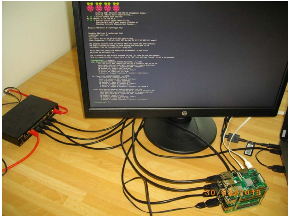
Figure 7. The Raspberry Pi3 will boot from the SD card, text output to monitor.
