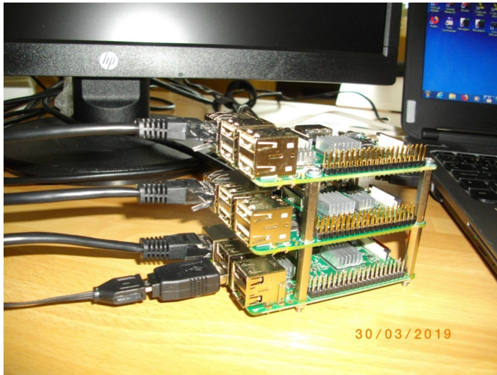
Figure 6. Raspberry Pi3, Arrowhead G4.0 clients on two ZynqBerry boards.
