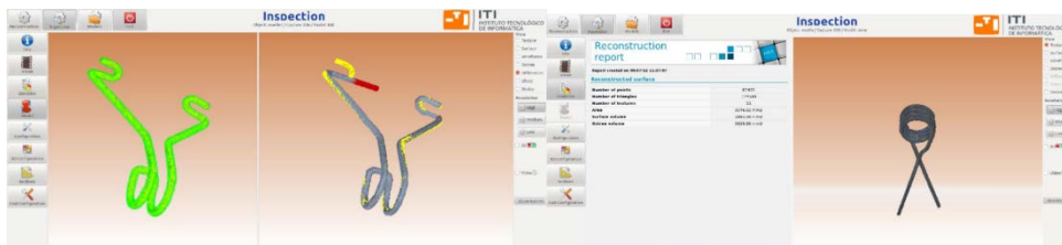
Figure 6: Comparison between actual produced part against CAD model
