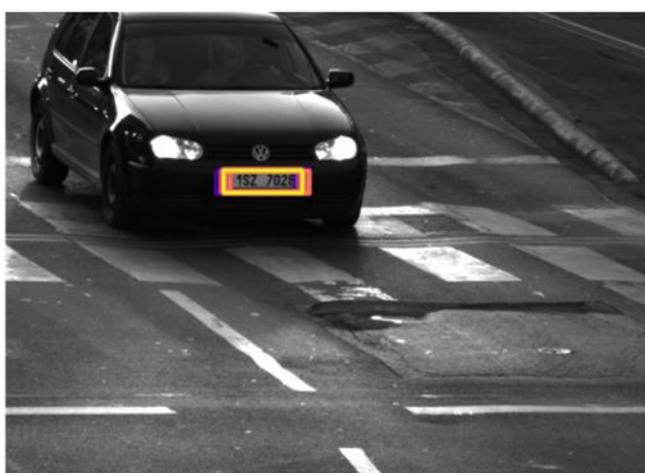
Figure 32: Example of detected license plates.
