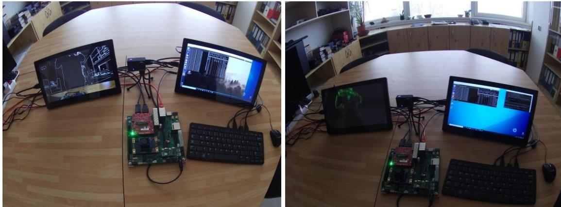
Figure 62: SW (Sobel and LK DOF) on the Zynq Ultrascale+ ZU15EG device.
